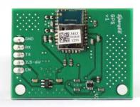
The GPSv1.0 is provided as a wide input range GPS development board based on the Antenova M10478 GPS module which contains a SiRFstarIV 9333 GPS chipset. Please see the M10478 datasheet for further specifications and features.
