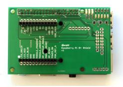
The ShieldRB+ is a shield or connecting board that connects the CELLv1.0 to the Raspberry Pi B+ without any additional wiring. It also provides LEDs for the CELLv1.0 status lines.
