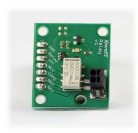
The RELAYv1.0 is provided as a wide input range relay board.
