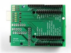
The ShieldAv1.0 is a shield or connecting board that connects the CELLv1.0 to the Arduino without any additional wiring. It also provides LEDs for the CELLv1.0 status lines.
